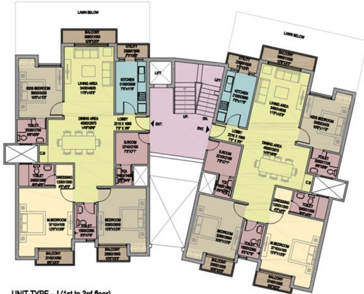
UNIT TYPE - J (1st to 3rd floor) SUPER BUILT UP AREA=1900 Sq.ft.
